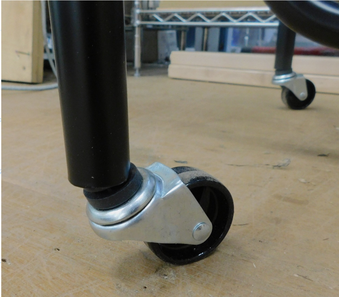
Picture 3: Castor after 180kg load view of the '44453 – Standard Clothing Rails – L 6ft x H 5ft'
